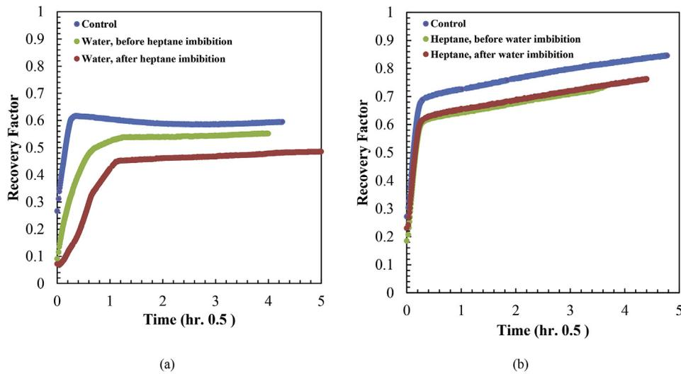
Fig. 1. The imbibition results: a) water Imbibition b) oil Imbibition.
