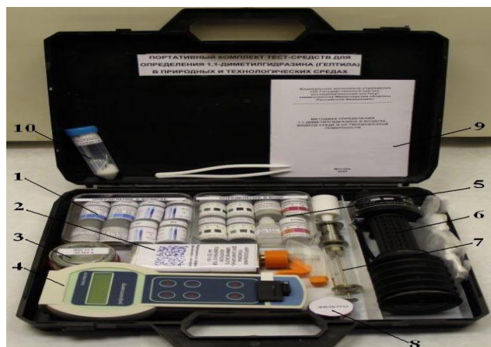
Fig. 1. Physical configuration of portable test kit intended for 1,1-dimethylhydrazine detection in the environment:
